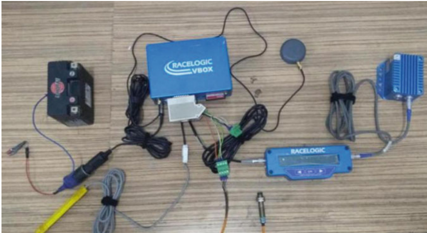
Fig. 4 Data logger connections
