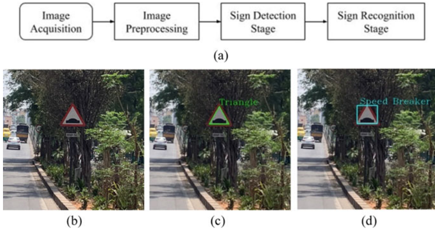
Fig. 1 a Methodology b input test image, c sign detection, d sign recognition
