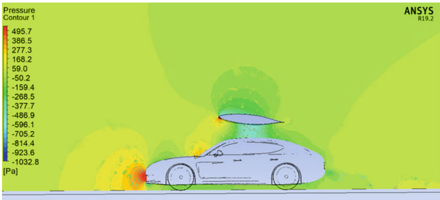
Fig. 6 Pressure plot of CFD model, car attached with wing
