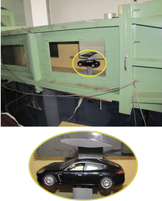
Fig. 2 The car body with the airfoil attached in the wind tunnel test
