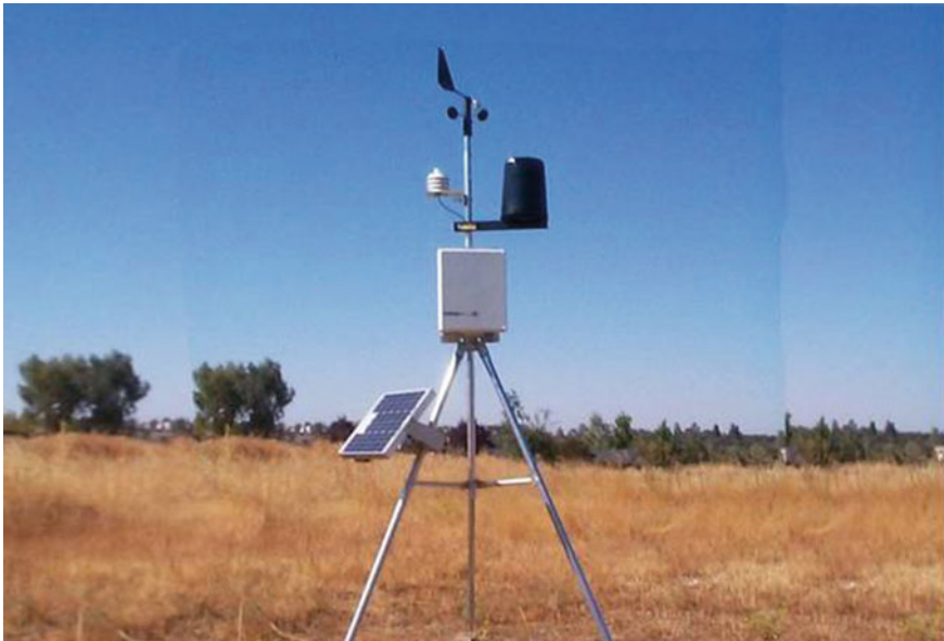
Fig. 5.18 Weather monitoring station and system, logics PowerAMR image courtesy of [48]
