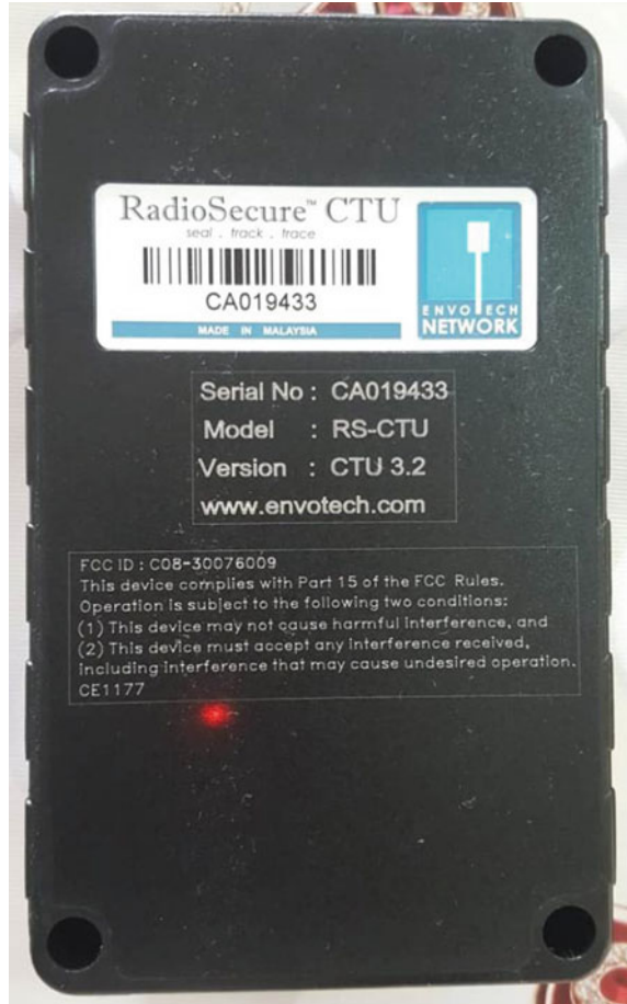
Fig. 13.2 RFID-based digital tracker (CTU) for COVID-19. Source Author
