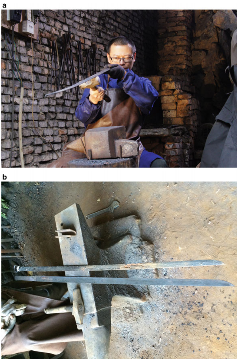
Fig. 7.33 Adjust the shape of dao to conform to the original Han dao
