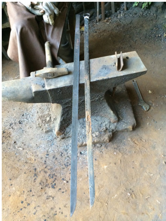
Fig. 7.28 Comparing the semi-finished dao with the ancient blade
