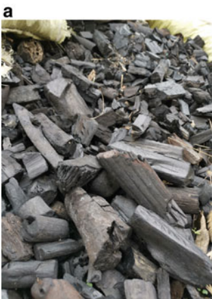
Fig. 7.4 White charcoal made from burnt Wugang oak. They are of great heat output and can burn for a long time
