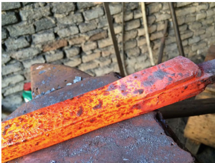
Fig. 7.26 The three-layer composite steel that was used for forging the blade
