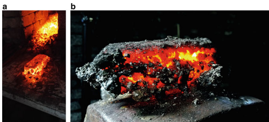
Fig. 7.23 The product of guan'gang , an amalgamation of cast iron and wrought iron
