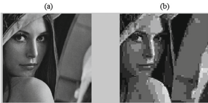
Fig. 4 Quantization effects on the 2D image. a Original 8-bits image and b 3-bits quantized image
