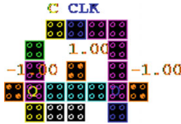
Fig. 6 Proposed level-sensitive ‘D’ flip-flop with reversibility
