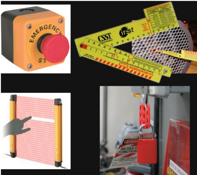
Fig. 14.5 Mitigation measures that can be applied to industrial robot cell (upper left, emergency stop; upper right, safety distance related to projectors; lower left, safety light curtain; lower right, lockout procedure)
