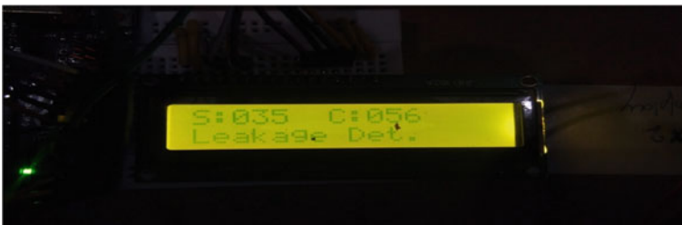
Fig. 5 LCD screen after leakage detection
