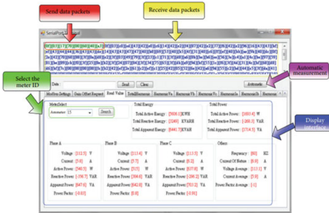
Fig. 4 Information interface for three-phase voltage and current and electrical energy
