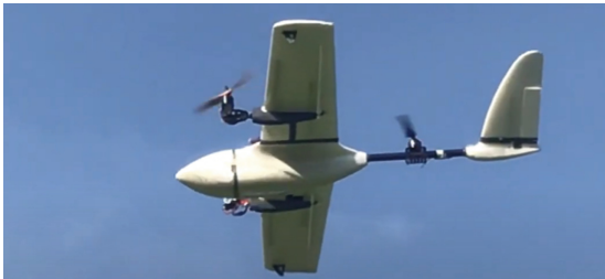
Fig. 8. A flying test of the Tilt Tri-rotor in hover mode
