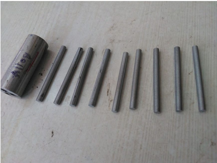
Fig. 1 Wear cut specimen using WEDM
