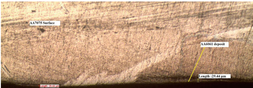
Fig. 6 Coating thickness of friction stir processed AA7075-T6 by AA6061-T6
