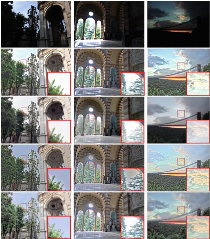
Fig. 3 Results of different tone mappers. From summit to foot: the bilateral filter, VAD method, LEP method, and ResNet model. Bilateral filter introduces halo artifacts at the edges across the tree in the summit image. Information are lost in case of VAD method. The local edge preserving filter method results are not quit natural look. ResNet model conserves the edge information
