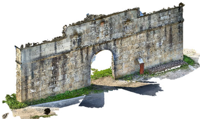
Fig. 4 Point cloud acquired with iPad Pro
