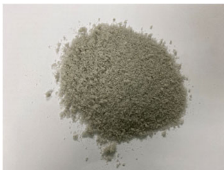
Fig. 1 Appearance of crushed polyurethane
