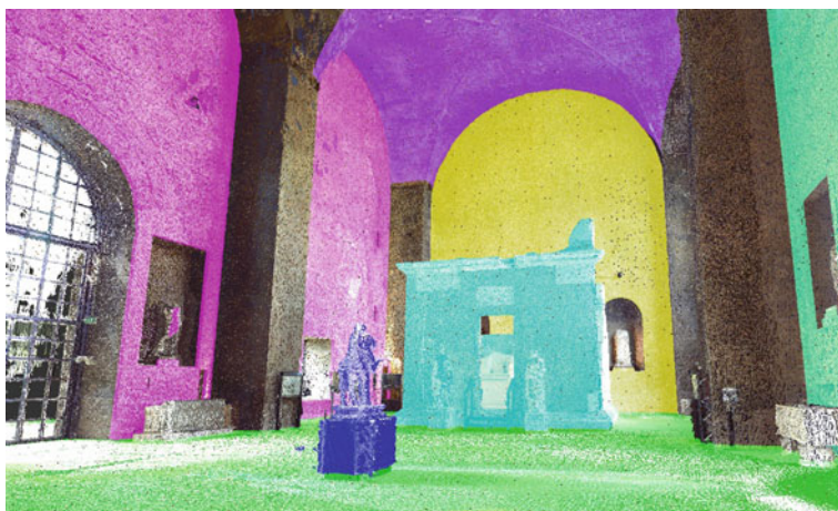
Fig. 9 Point cloud segmentation process represented by a color scheme
