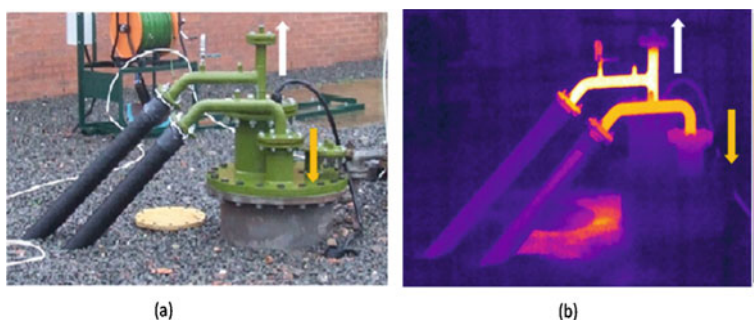
Fig. 8 Heat patterns in Markham (the arrows show the direction of water flow from and to the coal mine); Visual image (a) and Corresponding infrared image (b)
