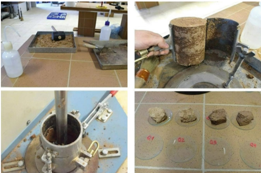
Fig. 9 Pictures show an example of the performance of a standard proctor test
