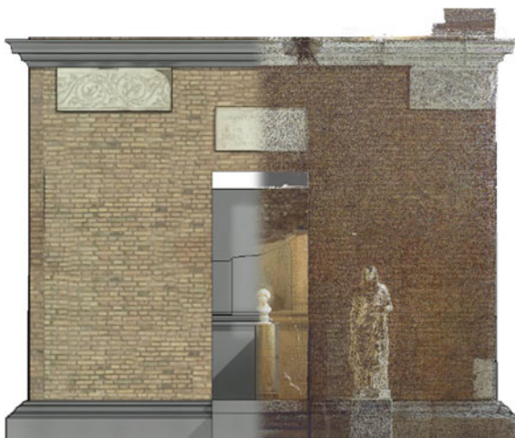
Fig. 8 Point cloud merged with BIM model for a visual benchmark
