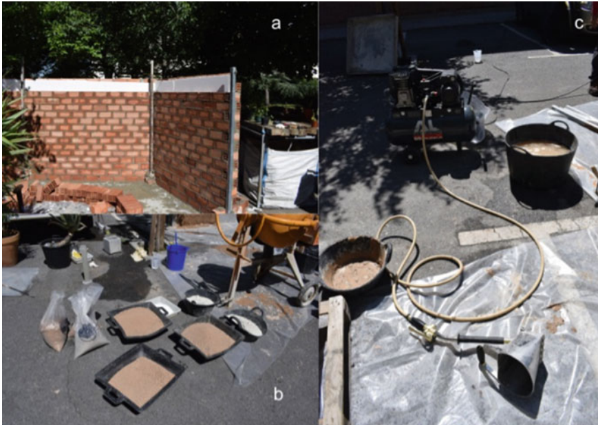
Fig. 13 a Ceramic brick factory wall that will serve as a support to project the mixtures. b Example of materials dosed by weight prepared for projection. c Tigre plaster sprayer plugged into compressor
