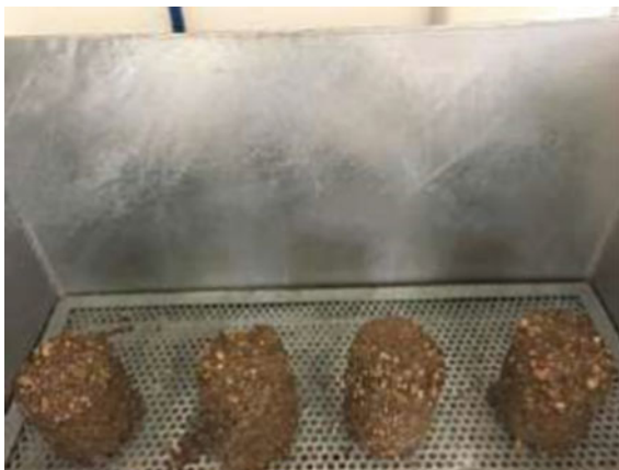
Fig. 12 Example of cylindrical samples compacted to standard proctor density placed in rain test machine
