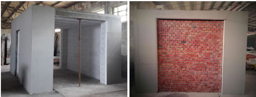
Fig. 1 Test chamber (left) and tested brick wall before installation of thermal insulation (right)
