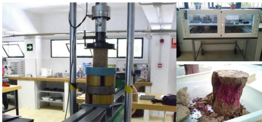
Fig. 11 Electric compression multi-test machine used (left). Forced carbonation chamber (top right) and sample after unconfined compression test and depth of carbonation test with phenolphthalein (bottom right)
