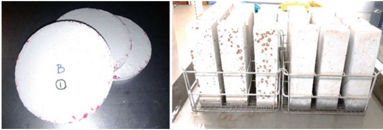
Fig. 2 Specimen permeability test (left); suction test (right)
