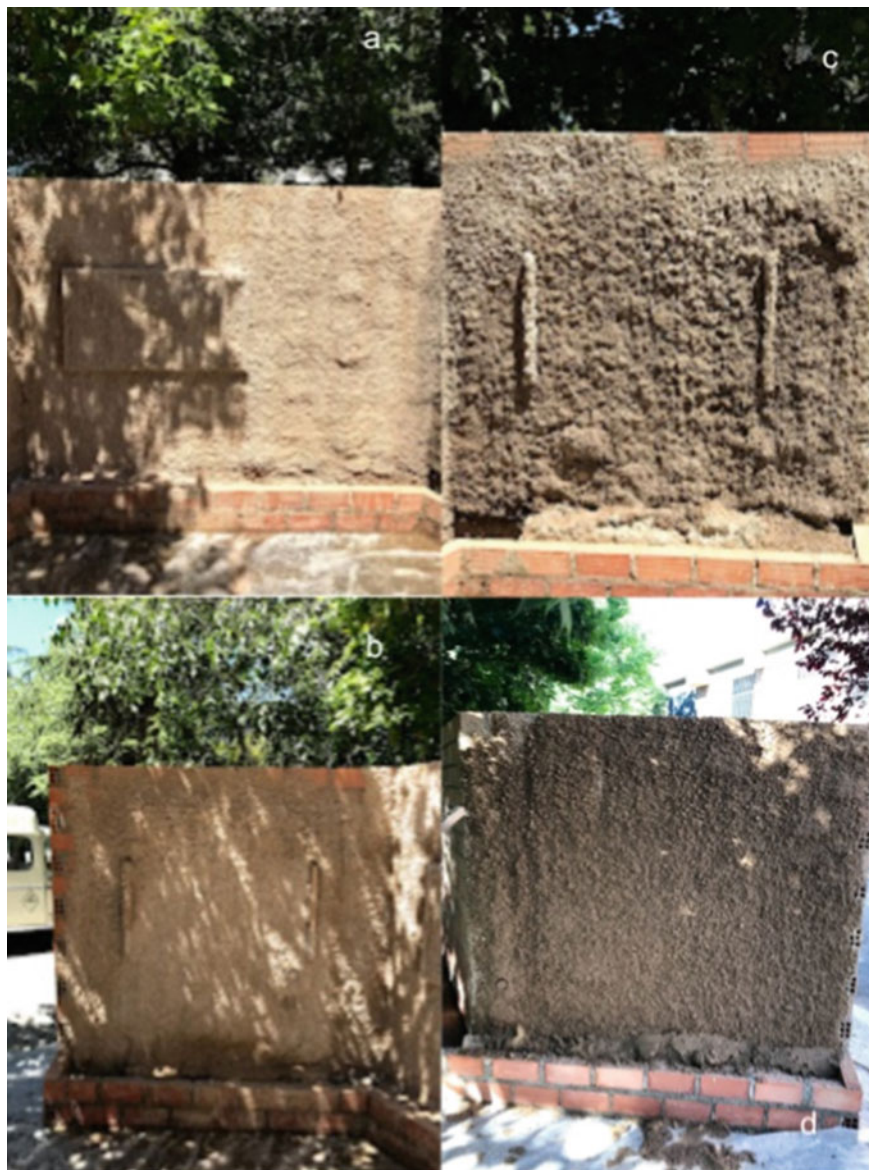
Fig. 14 Result of the projection of the different mixtures. a Earth + natural dolomitic aggregate + aerial lime + white cement. b Earth + recycled aggregate + aerial lime + white cement. c Earth + ecological enzymes + clay. d Earth + rubber powder and textile fibers + aerial lime + white cement
