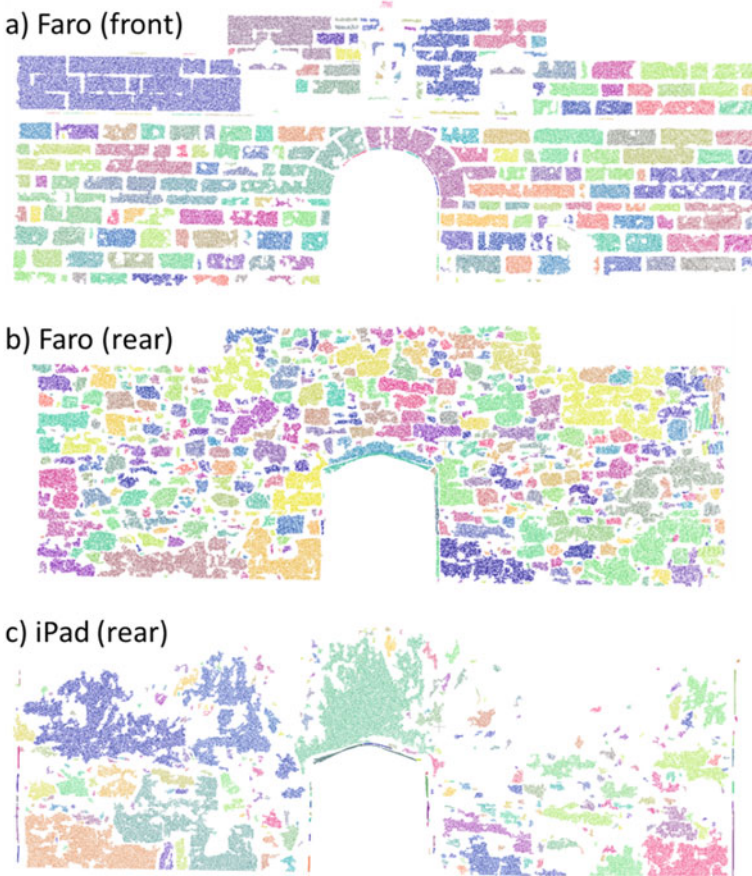
Fig. 9 Results of the application of connected components for the individualisation of stones. Individualised stones displayed in random colours
