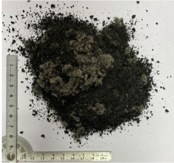
Fig. 7 Rubber powder and textile from tire waste
