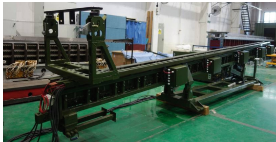
Fig. 4. Electromagnetic launch system for 100 kg fixed wing UAV
