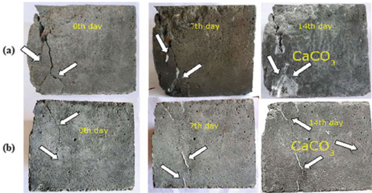
Fig. 14 Visual observations of BC 2 (a) cracks under FW and (b) cracks under WD
