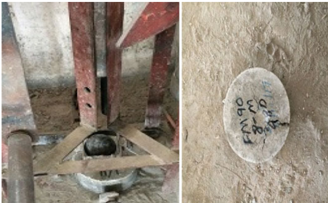
Fig. 9 Impact test setup and failure of impact specimen
