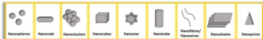
Fig. 12.3 Pictorial representation of some common shapes of nanoparticles
