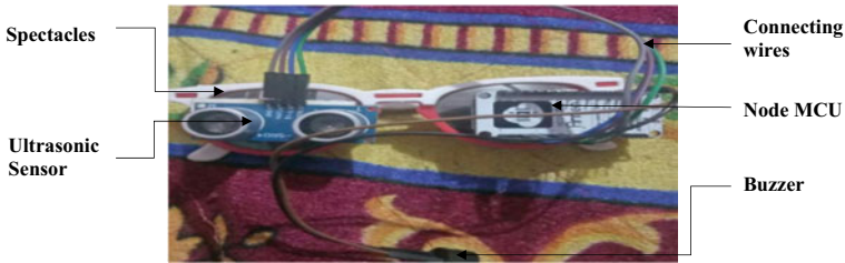
Fig. 6 Experimental setup of smart glass
