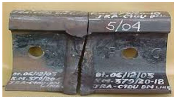
Fig. 1 Rail weld crack under a mix mode situation
