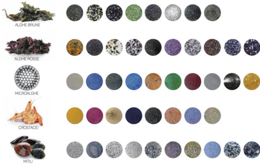
Fig. 9 Materials from the sea. Bioinspired material samples realized with raw materials of marine origin including algae, mussel shells, and shrimp, incorporated in biodegradable polymer matrixes. Credits: Francesco Amato, Clarita Caliendo (Design); Carla Langella (Scientific Design coordination); Mario Malinconico (Science material coordination)
