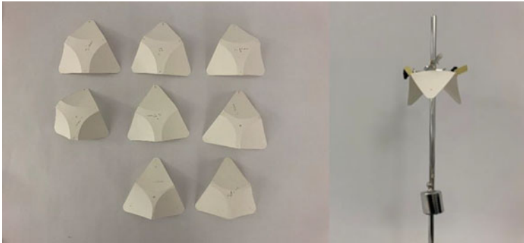
Fig. 22 Testing various curvatures with weights. © ArtBuild
