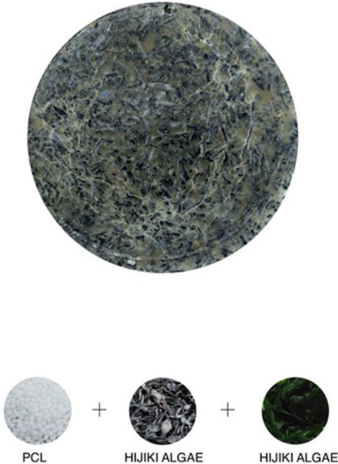
Fig. 10 Material sample composed of PCL and algae. Design: Francesco Amato e Clarita Caliendo. Design coordination: Carla Langella. Science material coordination: Mario Malinconico
