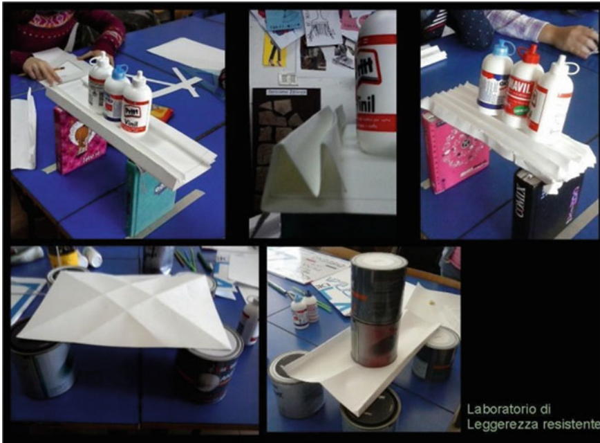
Fig. 14 Simple and intuitive resistance tests by bending cardboard surfaces
