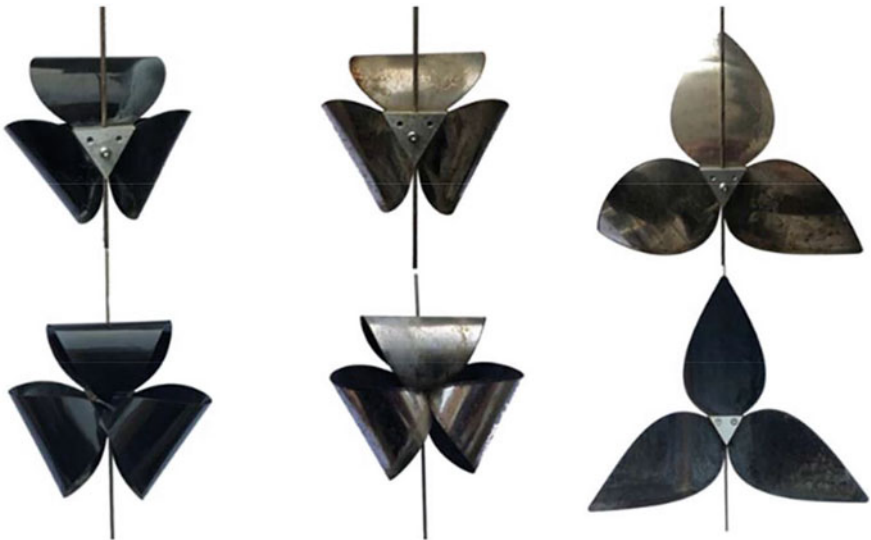
Fig. 11 Section of a mock-up model after outdoor anti-corrosion tests of 36 months (Left: painted TBM petals, Right: unprotected TBM petals). © ArtBuild
