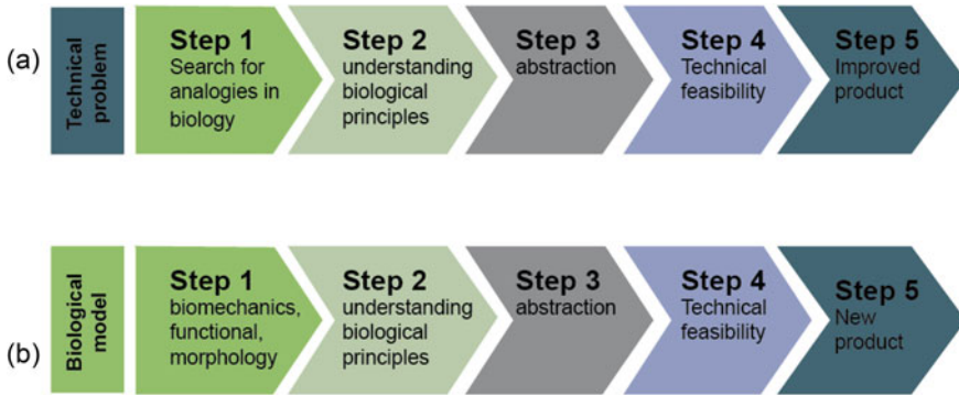
Fig. 4 Biomimetic design process. a Technology pull, b biology push. Adapted from ISO standard 2015:18,458
