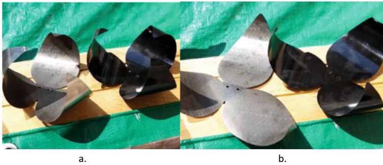
Fig. 12 Outdoor test aperture. Comparison of the movement of painted and unpainted TBM elements during the summer after being exposed for 10 s (a) and for 1 min on the left (b). © ArtBuild
