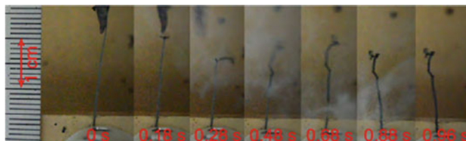
Fig. 34.29 Self-sustained combustion of composite fiber propellant
