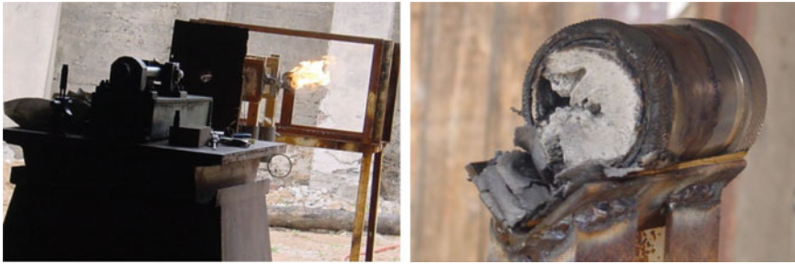
Fig. 40.6 Response status of 12.7 mm bullet impact test
