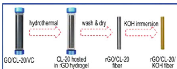
Fig. 34.11 Process of dimensional-limited hydrothermal preparation
