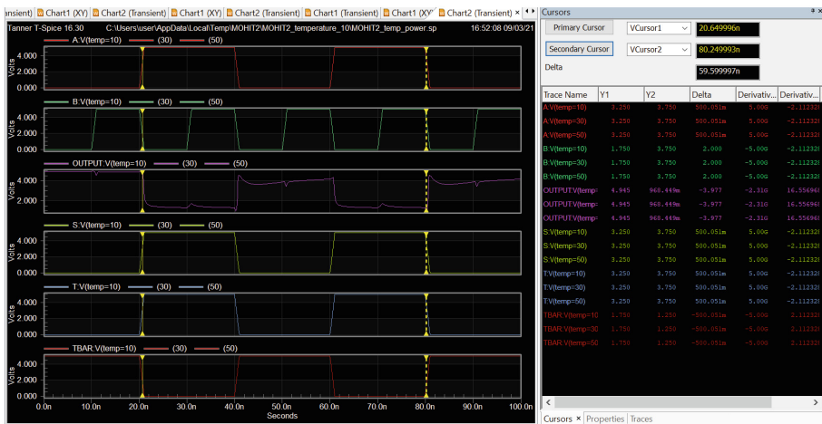
Fig. 7. Output waveform of 3T NOR gate with VS-MTCMOS technique at various temperature points
