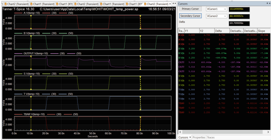
Fig. 4. Output waveform of NOR gate by pull down & pull up network with VS-MTCMOS technique at various temperature points
