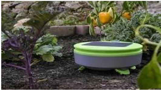
Fig. 2. These kinds of robots is used for killing the weed by using a sensor which is placed at the green position where it identifies weed and crop plan
