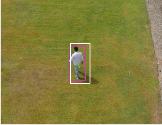
Fig. 9. Ground-truth box (pink), detection (white) and line between centers (green)
