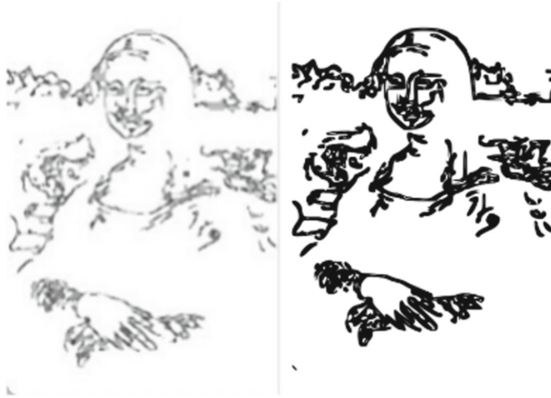
Fig. 6. The final output after MSED and vectorisation respectively
