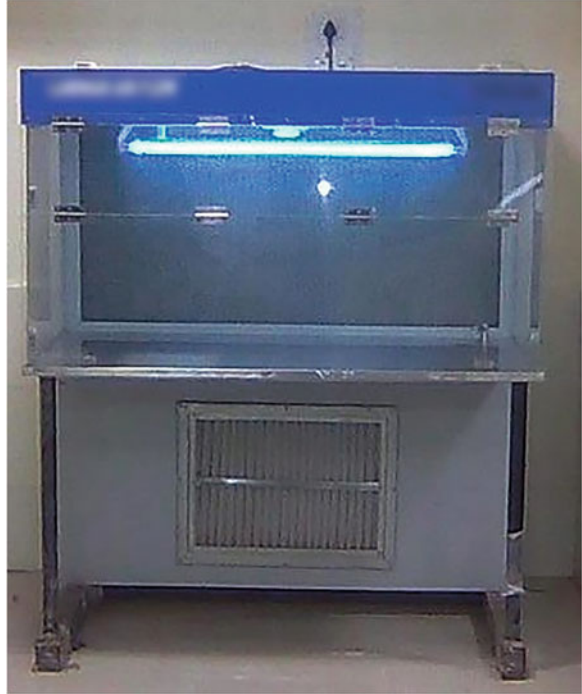
Fig. 1 Front view of a stainless steel laminar air flow (LAF)
