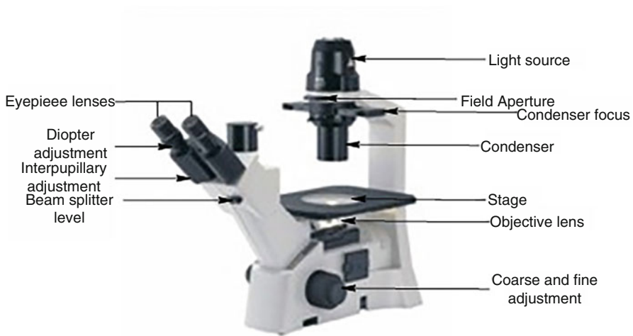
Fig. 6 Description of an inverted microscope
