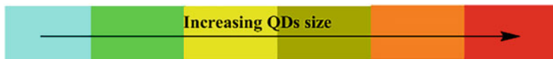
Fig. 15 An illustration of QD sorting in accord with size-emitting light of different colors excited simultaneously by a single-excitation wavelength
