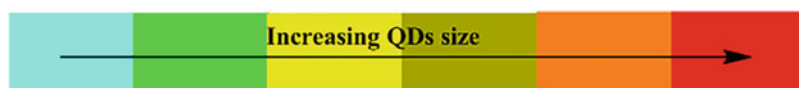
Fig. 15 An illustration of QD sorting in accord with size-emitting light of different colors excited simultaneously by a single-excitation wavelength
