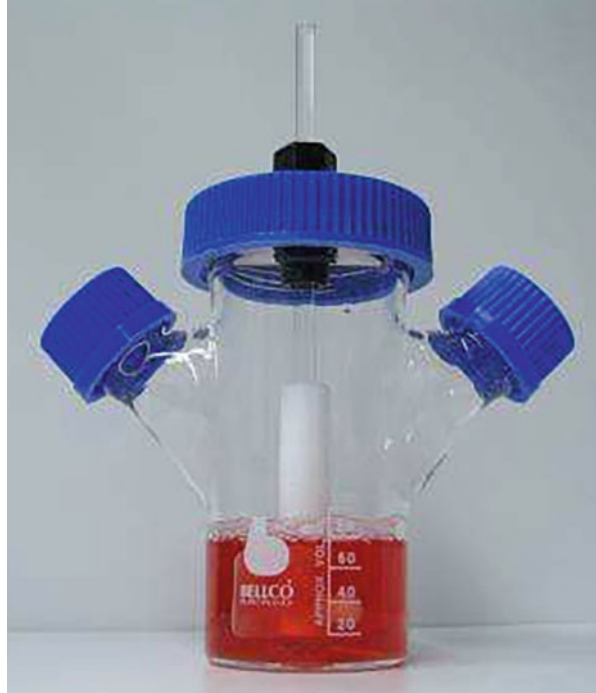
Fig. 2 Front view of a Spinner flask. (Image incorporated from our laboratory workable setup)
