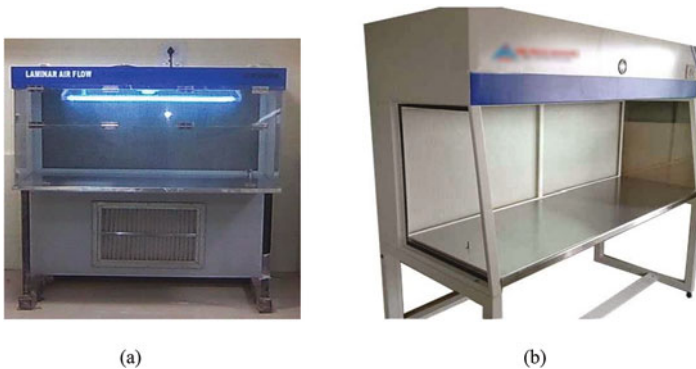
Fig. 2 Front (a) and side (b) views of laminar air flow (LAF) hood
