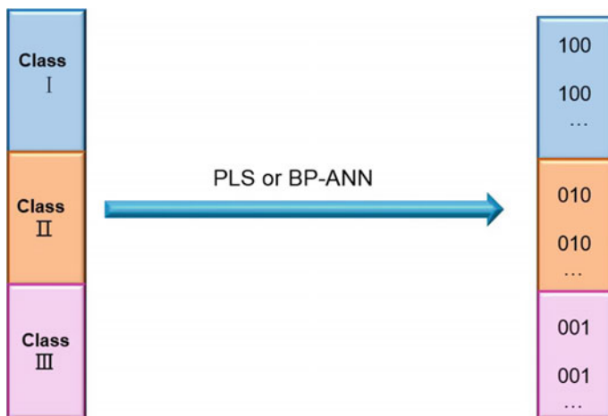
Fig. 12.15 Schematic diagram of regression method used for discriminant analysis of three classes of samples
