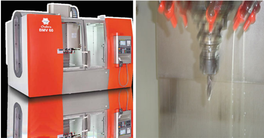
Fig. 2 Experimental setup for end milling operation
