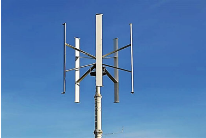
Fig. 1 The working model of vertical axis turbine view
