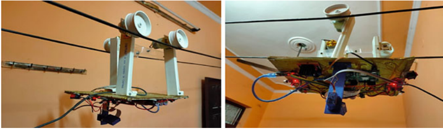
Fig. 2 Pictures of implemented rover moving on rope
