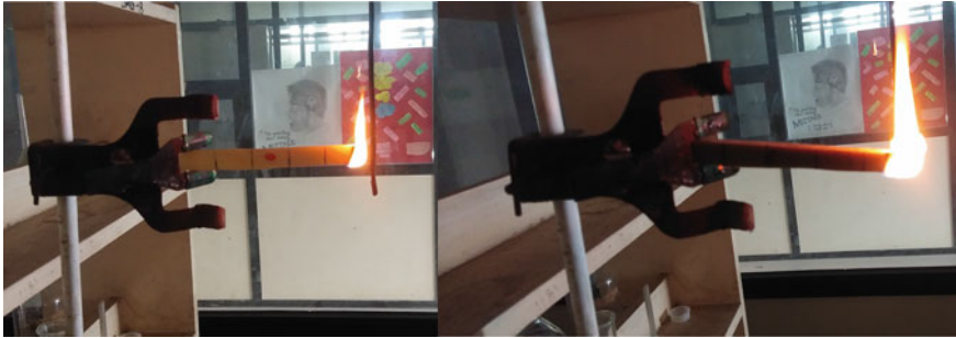
Fig. 1 Flammability sample testing of a horizontal specimen
