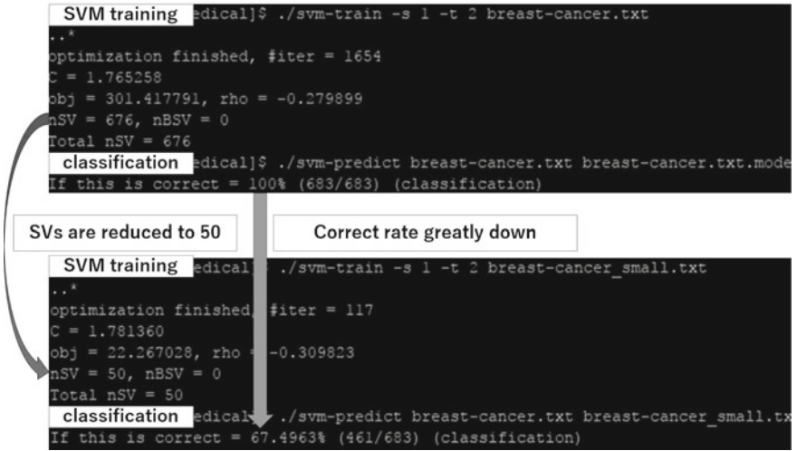
Fig. 3 Conventional SVM is applied for breast cancer diagnosis. When number support vectors is reduced, accuracy is going poor
