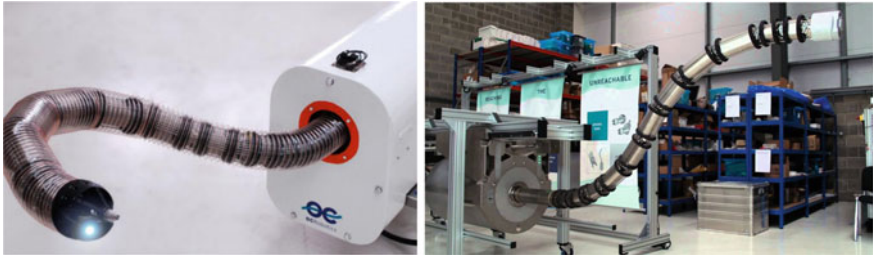
Fig. 1 Two examples of robotic trunk-like manipulators offered by Oliver Crispin Robotics Ltd. ( http://www.ocrobotics.com )
