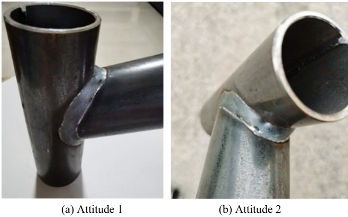
Fig. 6 Example of welding by manual demonstration method
