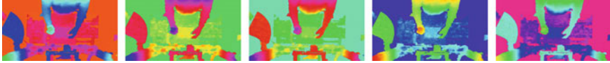
Fig. 5 Augmentation of a single depth image ( D_{\text{norm}}(u, v) ) using N = 5 colormap rotations resulting in five augmented images ( D_{\text{aug}, \phi(s_i)}(u, v, c) ) with randomly determined rotations ( \phi(s_i) ) from left to right: 21^\circ , 136^\circ , 162^\circ , 263^\circ , 325^\circ
