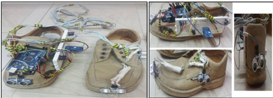
Fig. 4 Sensors attached to the shoes
