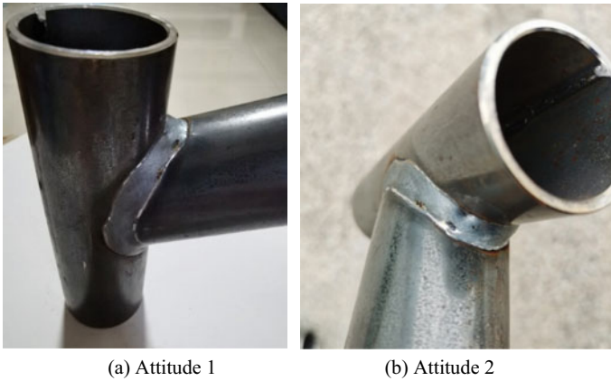
Fig. 6 Example of welding by manual demonstration method
