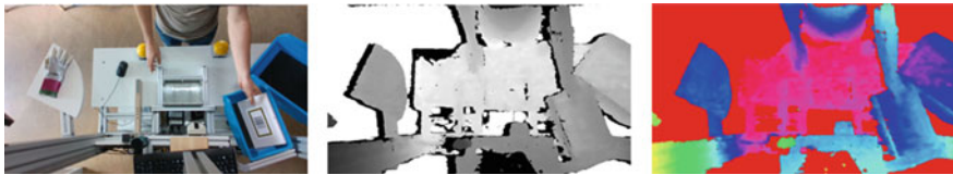
Fig. 2 Input samples. Left: RGB image. Center: Grayscale depth image ( D_{\text{norm}}(u, v) ). Right: Depth image encoded with HSV colormap ( D_{\text{hsv}}(u, v, c) )
