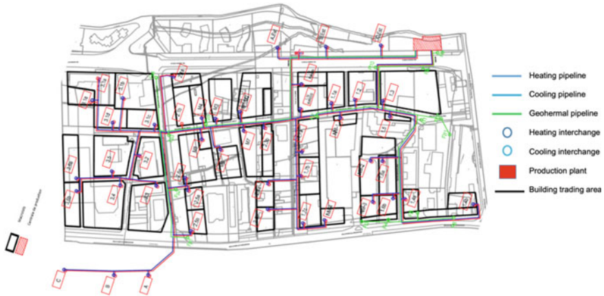
Fig. 64.1 Heating and cooling network with extraction and reinjection points for the new Meridia district (Source MNCA & IDEX)
