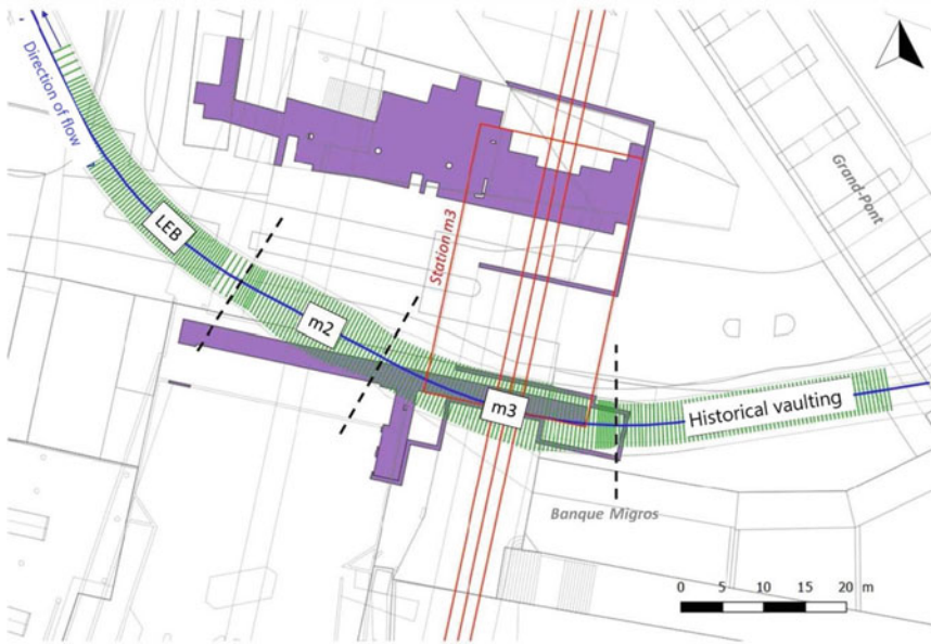
Fig. 61.1 Modifications of the Flon River vaulting at the Flon station. The historical works included modifications for the LEB and m2 metro lines, which are downstream of the planned m3. The historical vaulting remains upstream of the m3 and downstream of the LEB. The planned m3 tracks and the m3 Flon station (red lines) and the flow direction (blue arrow) are shown. Taken from Bourqui [4]
