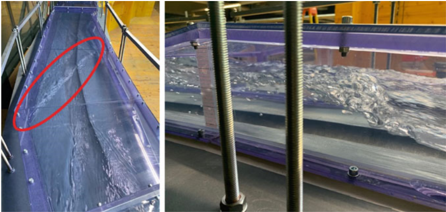
Fig. 61.13 Hydraulic phenomena on the physical model at Q = 17.9 \text{ m}^3/\text{s} (10 l/s on the model). A shockwave (red outline) on the m3 stretch was formed from left to right (left). The wave is caused by the sharp edge, which corresponds to the bend in the geometry. A hydraulic jump immediately upstream of the lowered m2 stretch was also seen (right)
