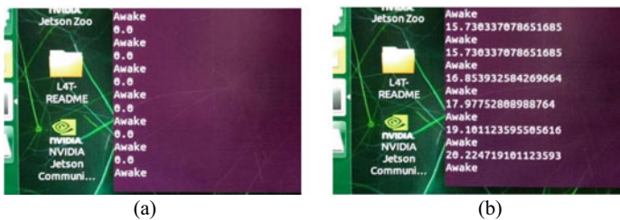
Fig. 7 a The PERCLOS value is not adding when the driver is on open eyes state and b The PERLOS value is adding when the driver is in close eyes state
