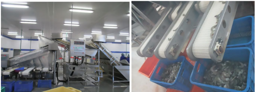
Fig. 2.52 Grading of shrimp with automatic grading machine
