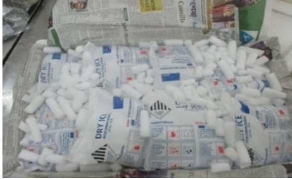
Fig. 10.7 Final layer of dry ice
