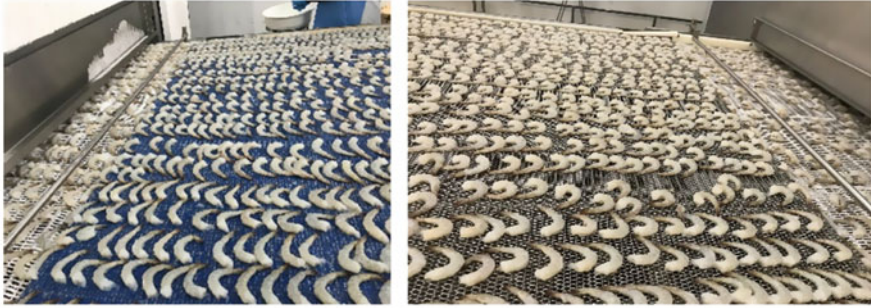
Fig. 14.5 A good practice, resulting no clumps and no hammering and no breakdown of clumps
