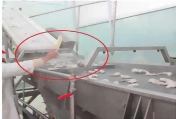
Fig. 14.3 Hammering on clumps to remove clumps
