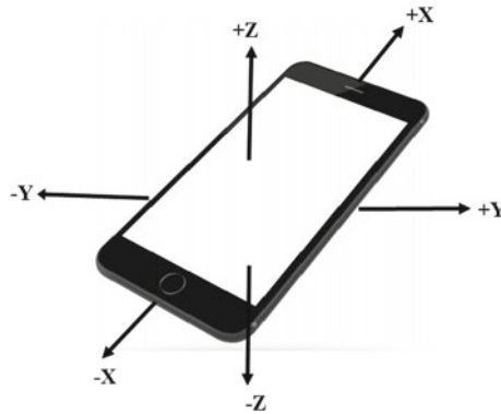
Fig. 3 The figure shows the x axis corresponds to the direction of travel, the y axis represents the horizontal axis movement and the z axis represents the vertical movement, i.e., measuring gravitational force. Any movement on the device applies force on the sensor which causes variations in the magnitudes on three axes. A static position captures only the gravitational forces across the z axis
