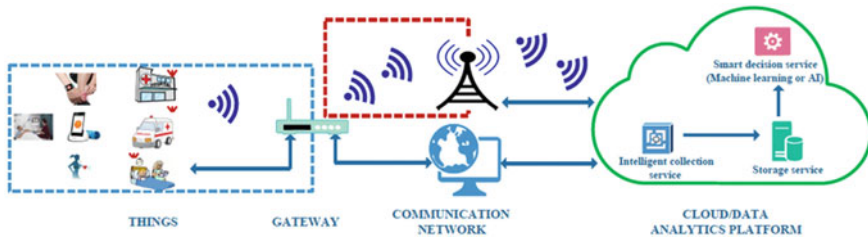
Fig. 2 Modern architecture of IoT-based smart health care (Alam et al., 2018)
