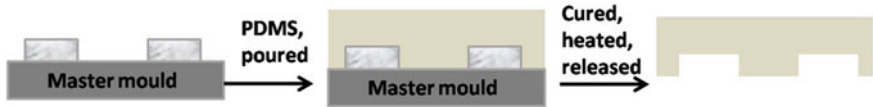
a: Schematic representation of the soft lithographic method of microfluidic device fabrication.
