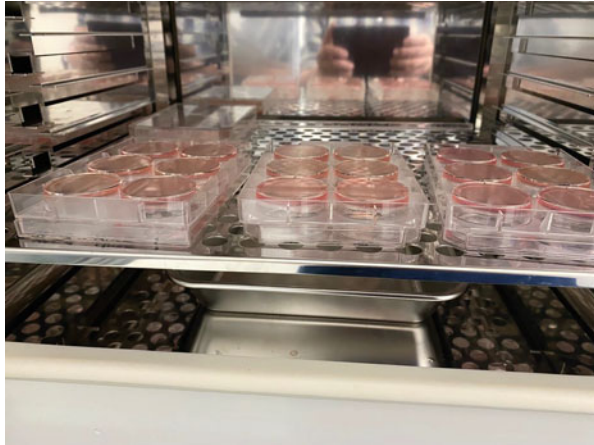
Fig. 4.12 Incubation of infected cells in plastic wells. The incubation is carried out in a CO 2 incubator
