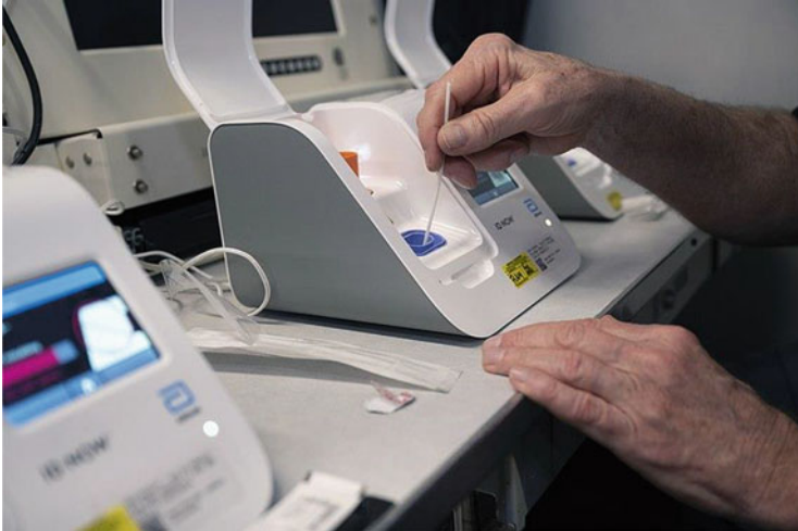
Fig. 10.4 Above is an example of nucleic acid testing using an Abbott Laboratories ID NOW device
