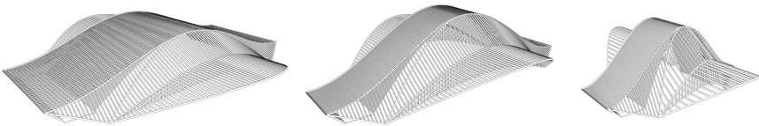
Fig. 7. Liège-Guillemins project: three possible variations of the model with different lengths, widths, and height for the central hangar.
