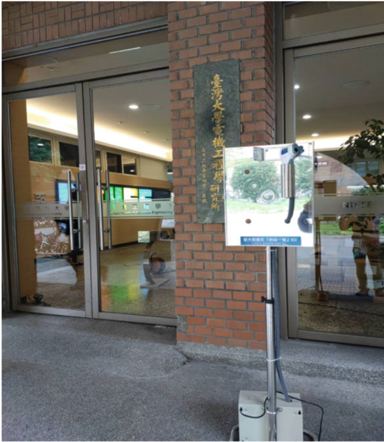
Fig. 9.6 The NTU Pandemic Prevention No. 1, an automated temperature-measuring device
