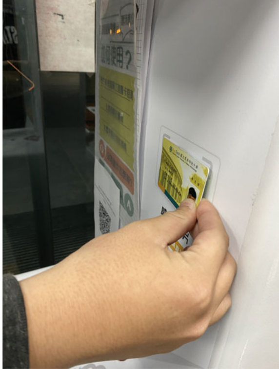
Fig. 11.6 Sensing the school ID card by the “Auto” inspection stand (Photographed by author)
