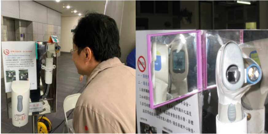
Fig. 9.7 The visitor does not need to touch any part of the forehead thermometer, as long as the forehead is close to the temperature measurement sensor. Temperature value can be seen from the L-shaped mirror
