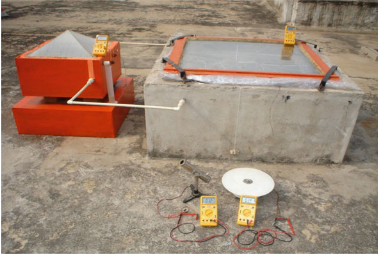
Fig. 1 Combined performance of Pyramid Solar Still (PSS) with Shallow Solar Pond (SSP)
