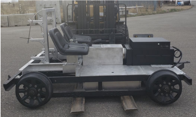
Fig. 7 Result of the retrofitted hydrail speeder
