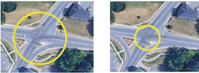
Fig. 3 Inscribed circle diameter of 55 m (left) and 27 m (right) on study intersection
