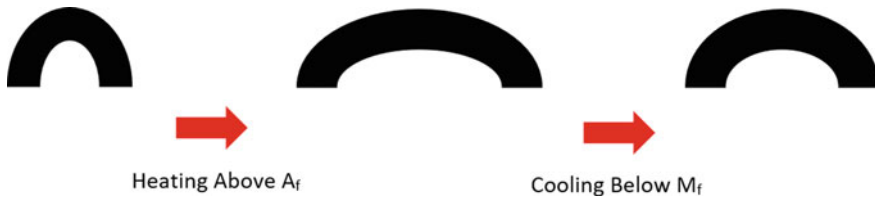
Fig. 1 Two-way shape deformation after irreversible deformation ( adapted from Karamichailidou [26])
