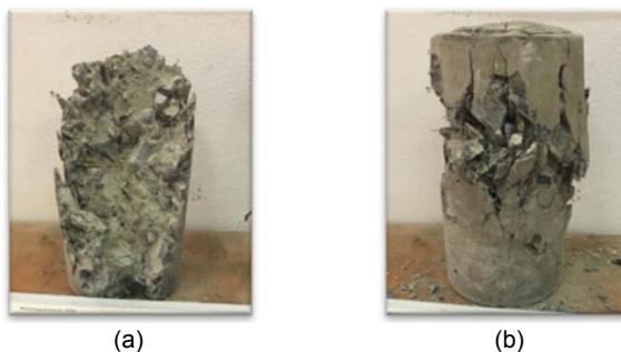
Fig. 3 Failure pattern of a control concrete cylinder with 0% fiber and 0% fly ash, and b FCF5F0 with 0.5% fiber and 0% fly ash at 56 days
