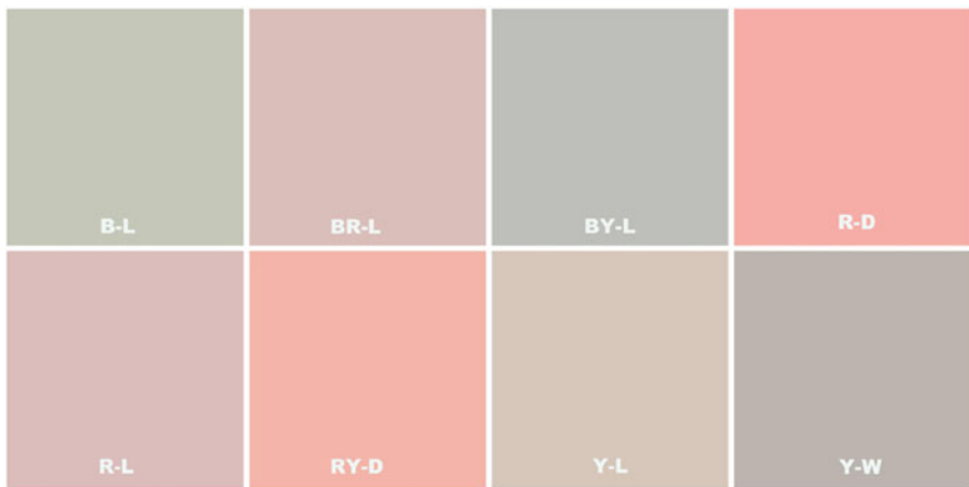
Fig. 5 Xylindein (blue-green), dramada (red), and the unknown yellow pigment from Scytalidium ganodermophthorum can be carried in natural oils, thereby eliminating the need for a solvent carrier. Image shows the color range available. B = xylindein, BR = xylindein + dramada, BY = xylindein + yellow pigment, R = dramada, RY = dramada + yellow pigment, Y = yellow pigment. L = raw linseed oil, D = Danish oil, W = walnut oil
