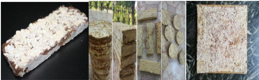
Fig. 6 Mycelium bio composite samples fabricated in different shapes and size
