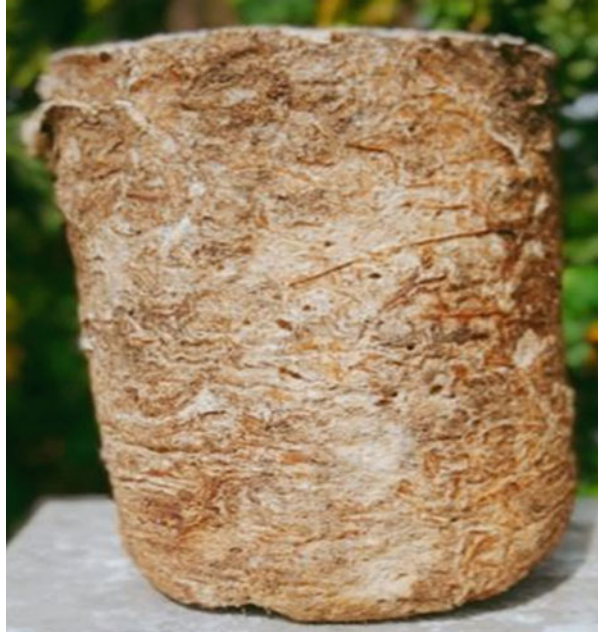
Fig. 4 Mycelium-sawdust bio composite foam
