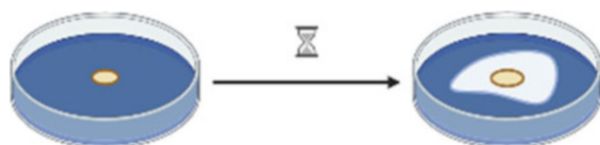
Fig. 2 Schematic representation of the DCPIP discolorization method performed in agar-based culture
