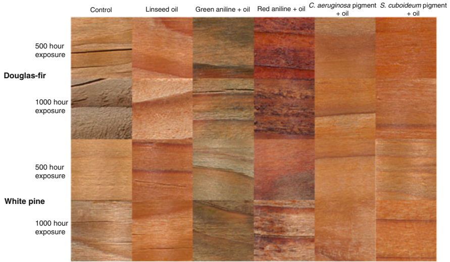
Fig. 4 Douglas-fir ( Pseudotsuga menziesii ) and white pine ( Pinus strobus ) wood treated with linseed oil, aniline dyes, or the pigment xylindein ( Chlorociboria species) / dramada ( Scytalidium cuboideum ) after an accelerated weathering test. The linseed oil mixed with the fungal pigments significantly decreased the cracking and greying of the wood. From Vega Gutierrez et al. (2021)
