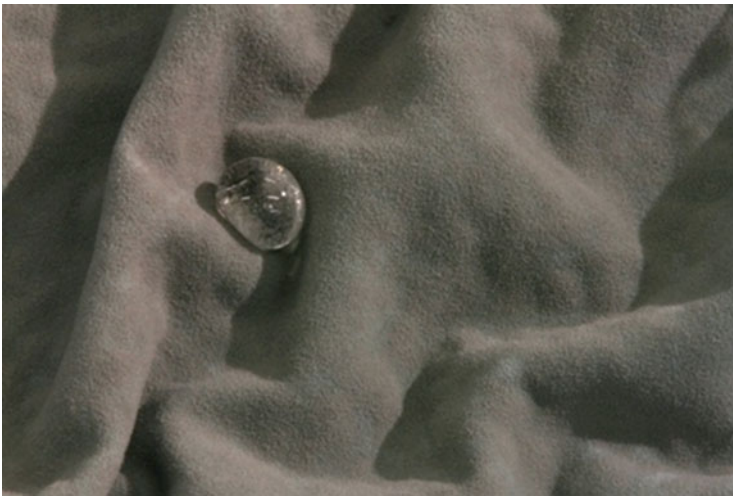
Fig. 21 Close up of the MycoCouture surface showing its hydrophobic properties (Park and Ivanova 2013). Image courtesy of Dr. Simon Park
