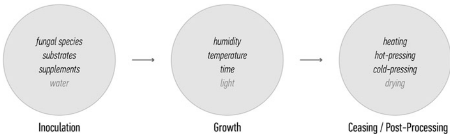
Fig. 1 Stages of MBC production and the factors affecting each stage
