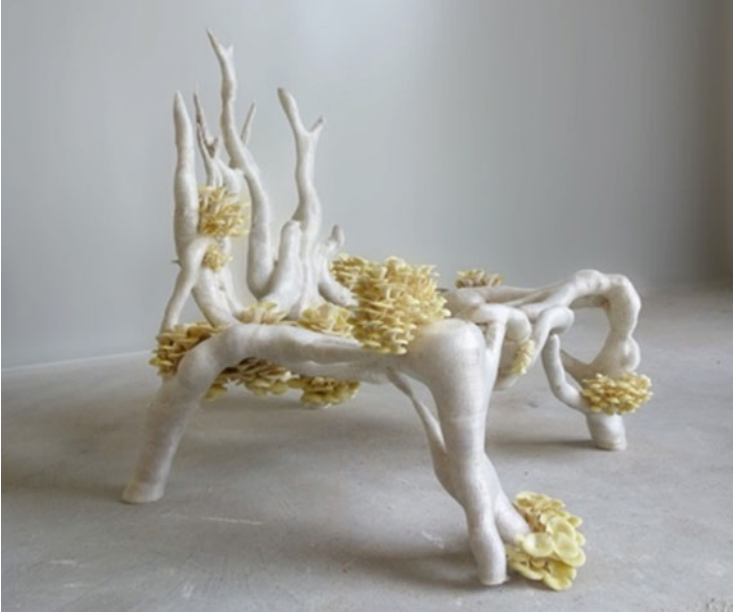
Fig. 13 Mycelium chair made using an adapted 3D printing process by Eric Klarenbeek. © Klarenbeek & Dros
