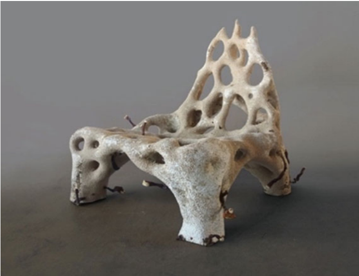
Fig. 14 Mycelium chair made using the improved 3D printing process, exhibited at the Centre Pompidu, Paris (2019). © Klarenbeek & Dros
