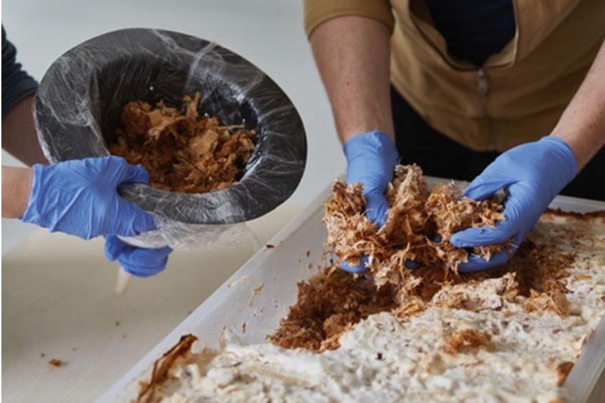
Fig. 24 Preparation of light shade formers filled with ‘myceliated’ wood for a second growth phase. © Petr Krejčí
