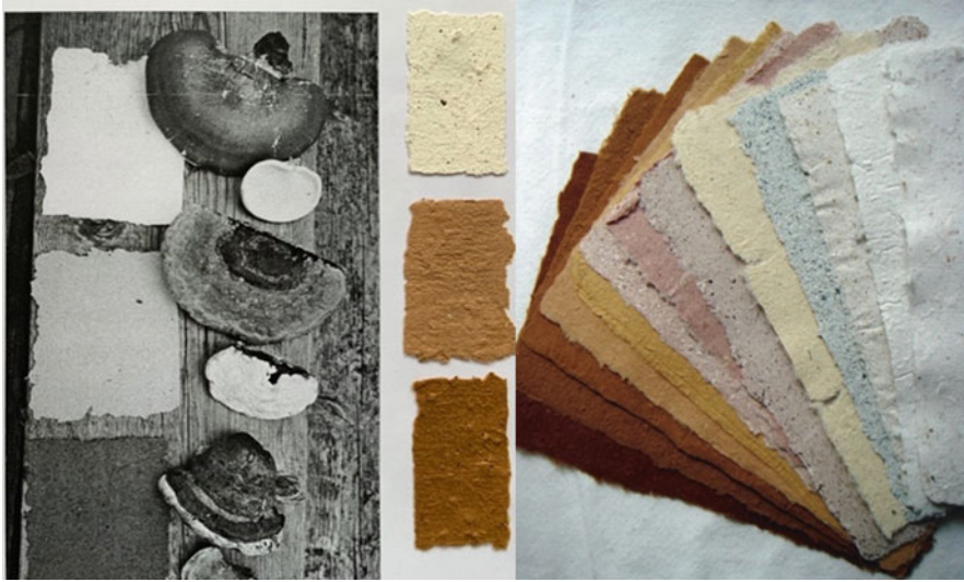
Fig. 6 Paper swatches produced from Piptoporus betulinus , Fomitopsis pinicola and Fomes fomentarius . © Johansson 2002 (left) and Mushroom paper created from various species © Johansson 2016 (right)
