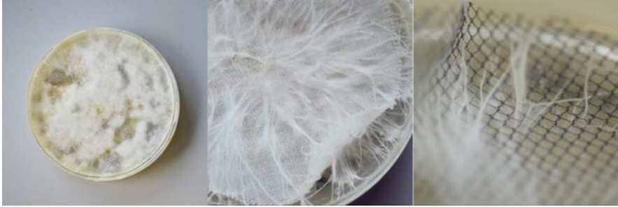
Fig. 19 Mycelial textile structures on netting and open weave cotton fabric. © Author's archive 2013
