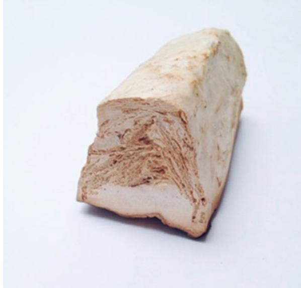
Fig. 25 A cross-section of moulded component illustrating different properties of the composite material. © Author's archive
