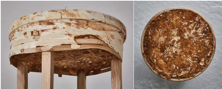
Fig. 27 Two mycelium stools made using green wood waste bound with mycelium to a wooden base and legs. © Petr Krejčí
