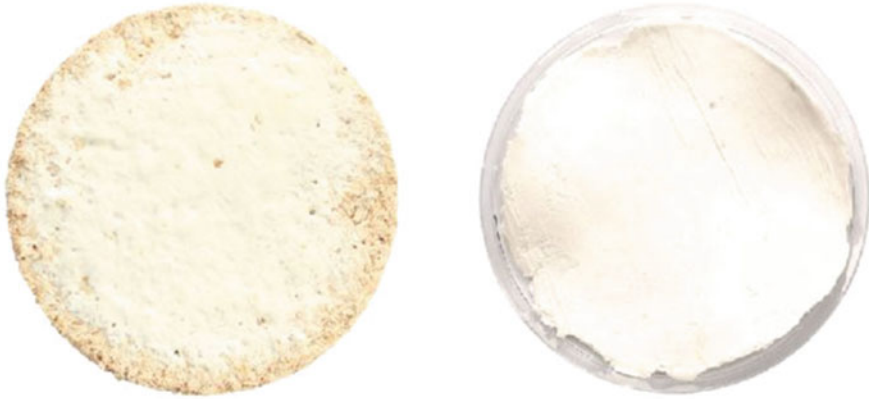
Fig. 1 Mycelium-based biocomposite (left) and pure mycelium (right) (Karana et al. 2018)
