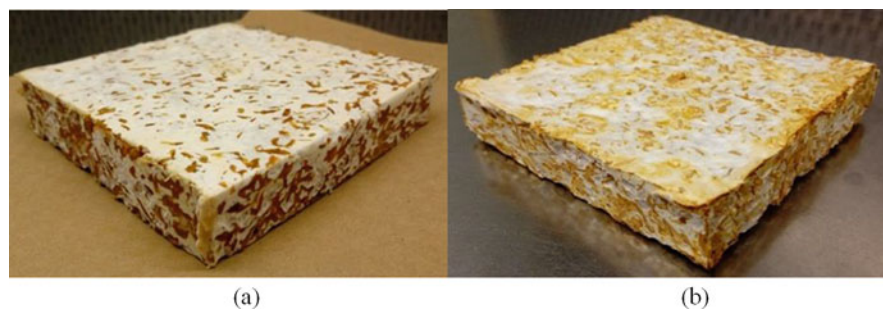
Fig. 3 Mycelium based composite material: (a) after growth, (b) dehydrated (Jones et al. 2017a, b)
