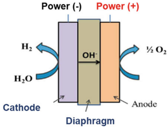
Fig. 8.4 Schematic diagram of the water electrolysis using the alkaline electrolyzer
